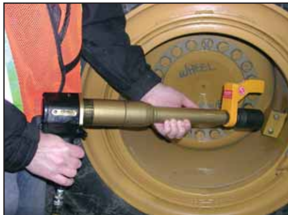
RAD 10GX (12818), 12" nose extension (14195), with reaction arm (13512)
